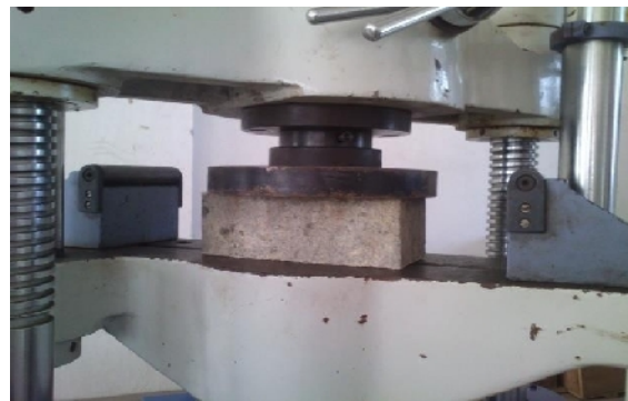
Fig 2. Testing of Brick
