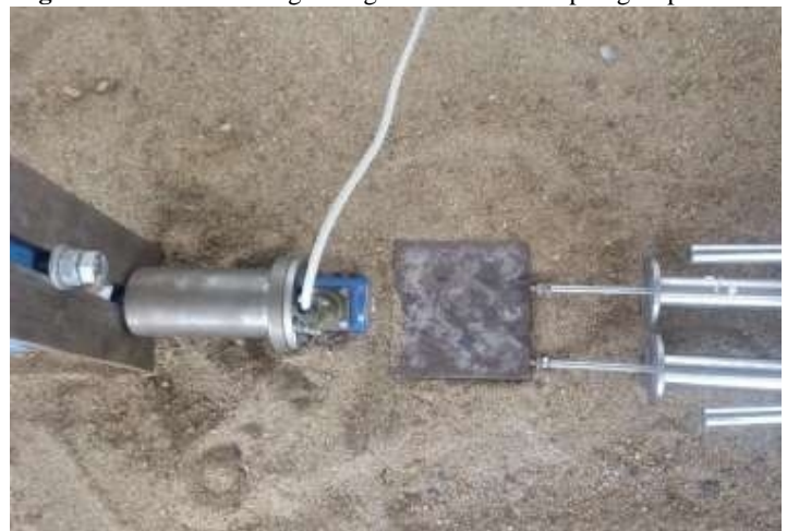
Figure 2. Lateral loading of positive batter pile group
