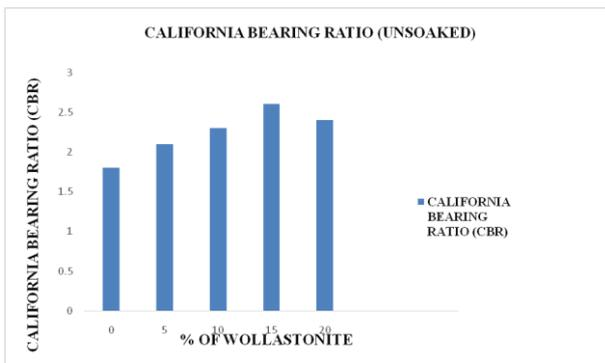
Figure 5: Comparison of various % of wollastonite and its california bearing ratio (CBR)
