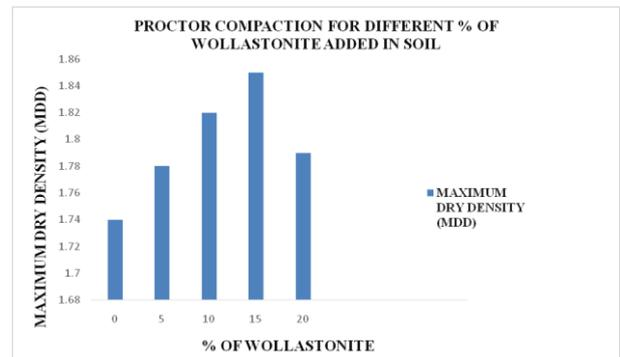
Figure 2: Comparison of various % of wollastonite and its maximum dry density (MDD)
