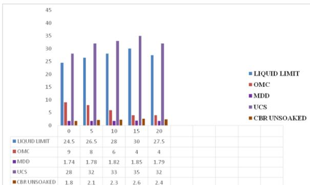
Figure 6: Overall comparison of various % of wollastonite with liquid limit, OMC, MDD, UCS and CBR value.
