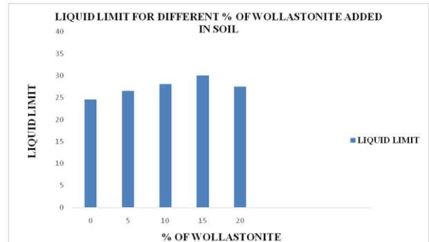
Figure 1: Comparison of various % of wollastonite and its liquid limit
