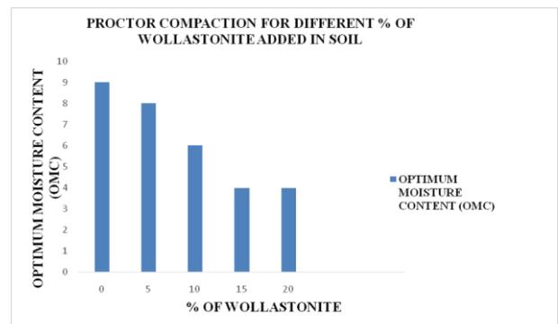
Figure 3: Comparison of various % of wollastonite and its optimum moisture content (OMC)
