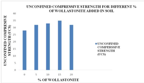
Figure 4: Comparison of various% of wollastonite and its unconfined compressive strength (UCS)
